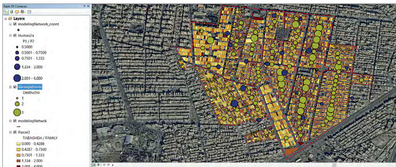
Figure 2: Input data illustrated in GIS to use in the DMCsim for District 17 of the city of Tehran, Iran simulation.
