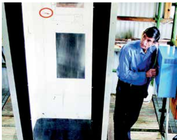
Dr Peter Ellis demonstrates how the vertical wind tunnel allows firebrand samples (circled) to be burnt at their terminal velocities in the laboratory, as though they were actually in flight.
