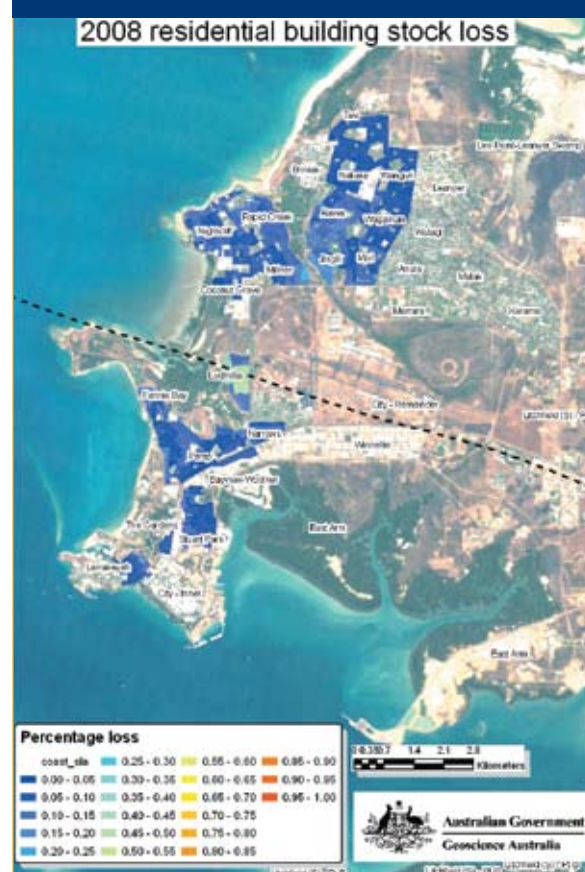
Figure 5: Estimated mean residential building stock loss (% RC) for Darwin in 2008 using the meshblock methodology.
