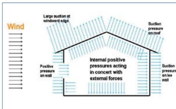
Figure 3: Wind forces with a dominant opening in windward wall
