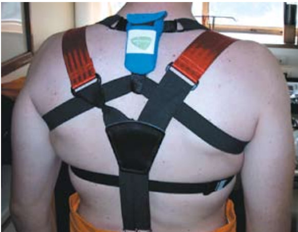
Figure 4: Portable global positioning system (inside blue pouch), heart rate, and activity monitors (connected to black horizontal strap) enable measurements of work patterns and energy expenditure during bushfire suppression without disrupting firefighter's work.
