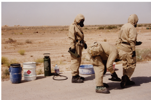
Detection/monitoring personnel for contamination at decontamination line, using chemical agent monitor (CAM) and AP2C monitor. Chemical decontaminant in the background
