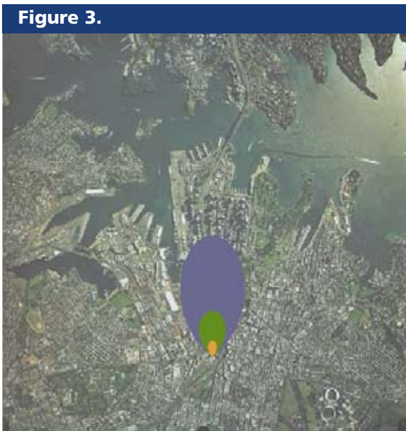
Figure 3: The defined regions represent various ground contamination levels (GCL) from the same scenario used in figure 1. The red represents GCL of greater than 100 kBq per m 2 , the green represents GCL of greater than 10kBq per m 2 , and the blue represents GCL of greater than 1 kBq per m 2 . Photograph © Department of Lands (2004).
