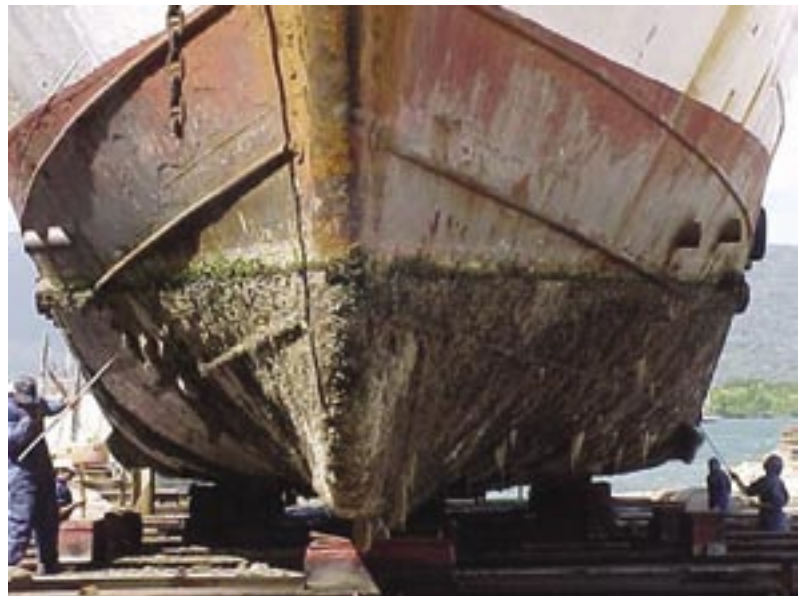
Defouling of an international trading vessel on a Cairns slipway Photo courtesy of Queensland Environment Protection Agency
