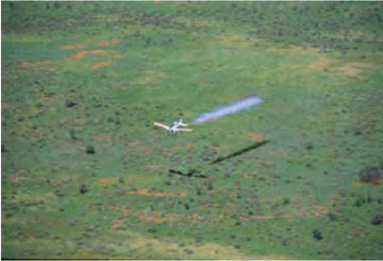
APLC contracted spray aircraft operating 'smoke' generator to assist determination of application drift risk [Courtesy: Randy Larcombe]
