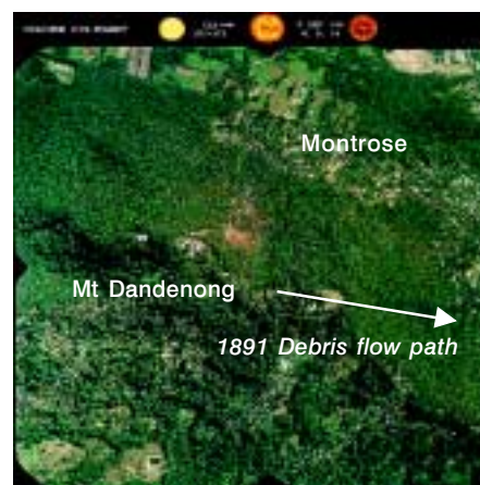
Figure 1: the Montrose landslide 1891 – 30,000 cubic metres of earth and rock moved down the slope at approximately 40km per hour.
