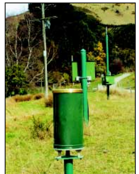
Figure 3: Telemetered rain gauge site at Blandswood
